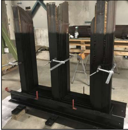
Core legs sprayed with dielectric varnish and then clamed
