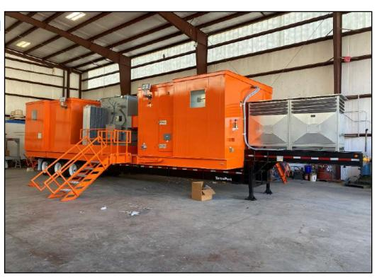
This is an AMR PEMCO Mobile Substation
