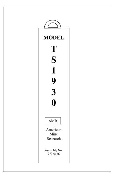
The AMR Tilt Switch is a simple yet versatile unit to sense material levels both underground and in surface operations. The TS-1930 is potted to increase its durability. It is designed to be hung vertically, using the attached eyehook. If it tilts more than 30 degrees in any direction, the normally closed mercury switch will open, breaking a control or sense circuit. The switch is rated for 120 VAC at 12.5 Amps
