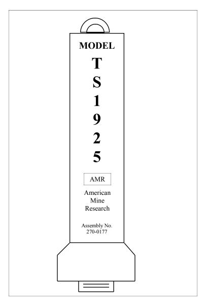
The AMR Tilt Switch is a simple yet versatile unit to sense material levels both underground and in surface operations. The TS-1925 is potted to increase its durability. It is designed to be hung vertically, using the attached eyehook. If it tilts more than 15 degrees in any direction, the normally closed mercury switch will open, breaking a control or sense circuit. The switch is rated for 120 VAC at 12.5 Amps
