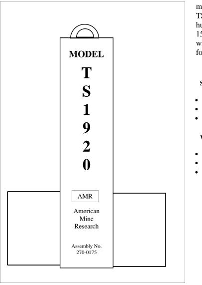
The AMR Tilt Switch is a simple yet versatile unit to sense material levels both underground and in surface operations. The TS-1920 is potted to increase its durability. It is designed to be hung vertically, using the attached eyehook. If it tilts more than 15 degrees in any direction, the normally closed mercury switch will open, breaking a control or sense circuit. The switch is rated for 120 VAC at 12.5 Amps
