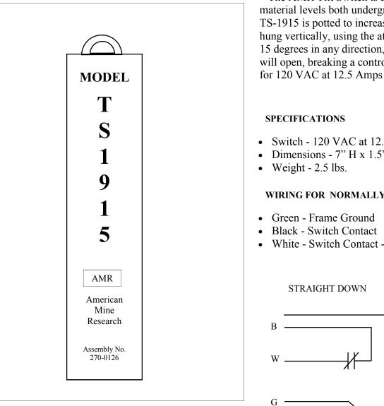
The AMR Tilt Switch is a simple yet versatile unit to sense material levels both underground and in surface operations. The TS-1915 is potted to increase its durability. It is designed to be hung vertically, using the attached eyehook. If it tilts more than 15 degrees in any direction, the normally closed mercury switch will open, breaking a control or sense circuit. The switch is rated
