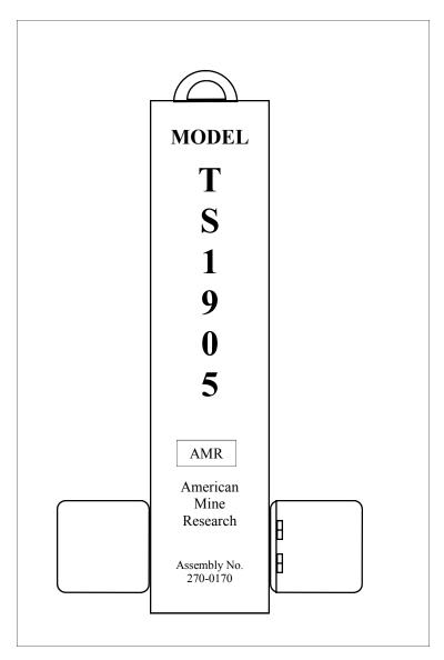
The AMR Tilt Switch is a simple yet versatile unit to sense material levels both underground and in surface operations. The TS-1905 is potted to increase its durability. It is designed to be hung vertically, using the attached eyehook. If it tilts more than 30 degrees in any direction, the normally closed mercury switch opens the units internal relay, providing normally open contacts. The switch is rated for 120 VAC at 7 Amps
