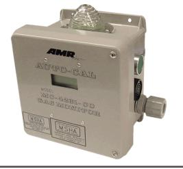
Data line connected CO monitor with high visibility LED and audible alarm. One compact surface mount PC board for sensor and communications with a wide range four-digit display. Is able to be calibrated without removing cover with non-intrusive sensor test and calibration with automatic surface reporting.
